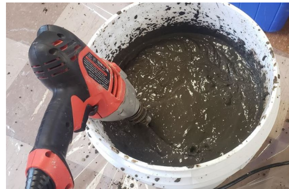
Homogenization of sediment using a mixing paddle attached to an electric drill
