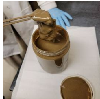
Polyethylene sheet retrieval after 28 days
