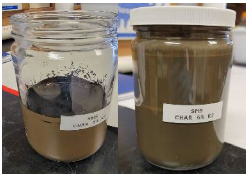
Dredged sediment with added amendment materials
