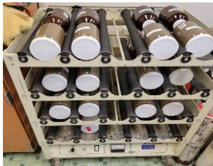
Dredged sediment samples on the roller for equilibrium study
